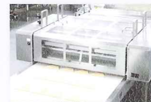
Two types of Turners: Super High Speed Turner and High Speed Turner. Super High Speed Turner-Max. 100pcs./min./row. High Speed Turner-Max. 50pcs./min./row.
