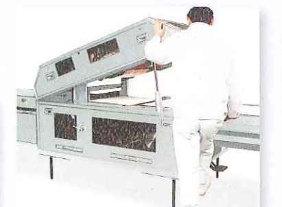
The Molder Section opens simply by stepping on the pedal.
